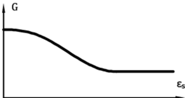
Figure 6: Curve describing the loss of stiffness of shear modulus
