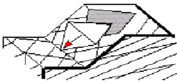
Translation on the polygonal slip surface
